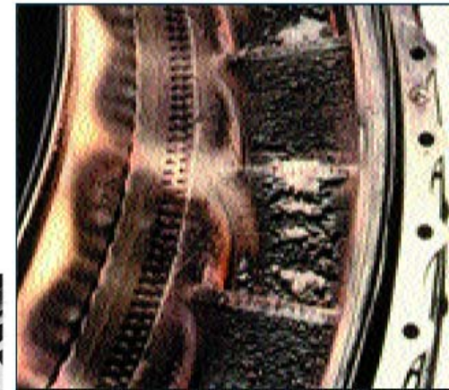
Figure 5. Sketch of deposits on stage-1 HPT nozzle guide vanes, based on borescope inspection of engine 1.
