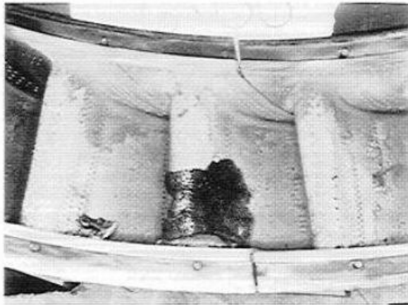
Figure 3. Dark, glassy deposits of remelted volcanic ash on leading edge of stage-1 high-pressure-turbine (HPT) nozzle guide vane (NGV).
