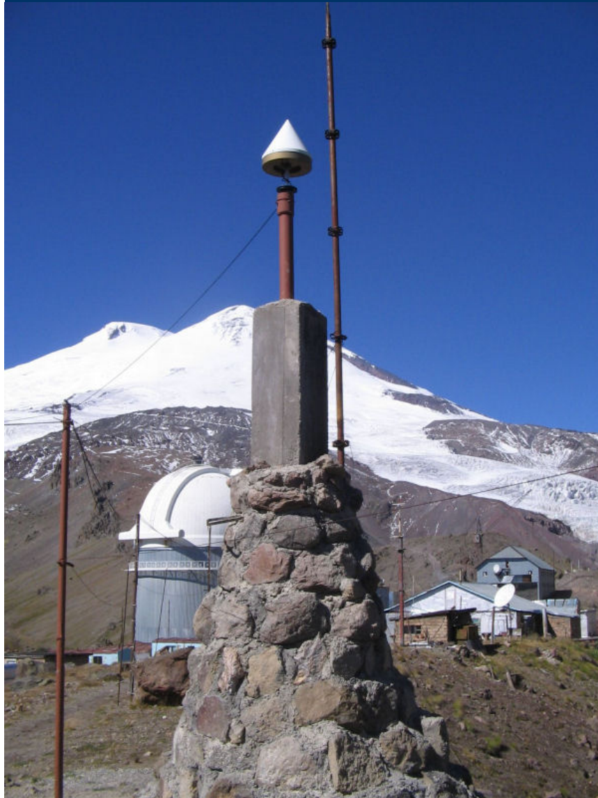
The TRSK station (GPS/GLONASS) of the Regional Northern Caucasus network [Milyukov, 2010], Terskol Peak, 3150 m, 3 km from the Elbrus volcano.
